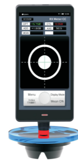
Step4:测量近光和远光区的度数 Step4:measure far and near view power
